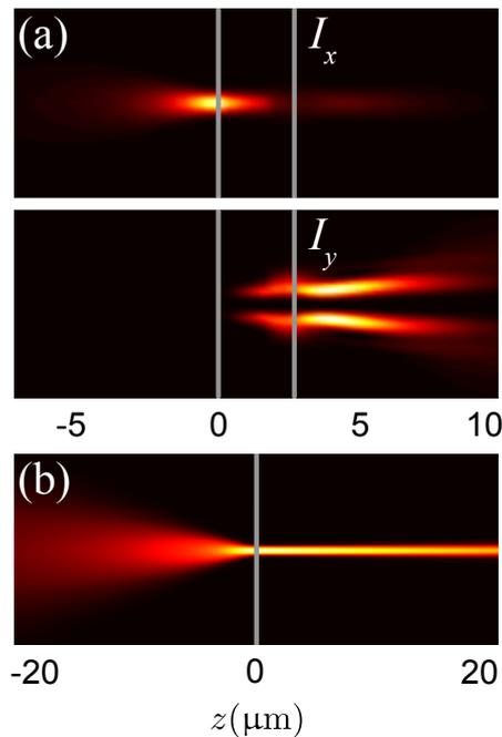
**Figure 1:** Influence of spatial dispersion on beam propagation. Polarization conversion is shown in (a) and diffraction compensation in (b).
