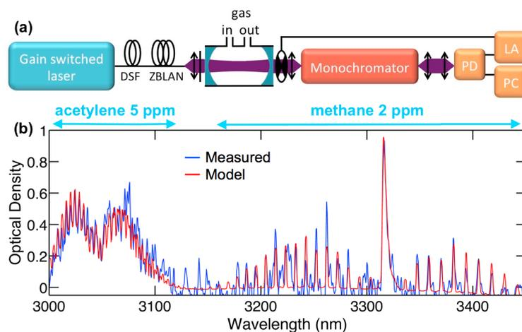
Figure 1: (a) Experimental setup. (b) Comparison between the measured and modeled absorption lines of 5 ppm of acetylene and 2 ppm of methane simultaneously in the cavity.
