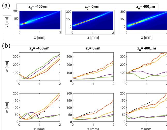
Fig.1. (a) Evolution of a 5 mW extraordinary-polarized beam in the plane  $yz$ . (b)  $w=w(z)$  curves for  $w_0=2$   $\mu\text{m}$  (top), and  $w_0=4$   $\mu\text{m}$  (bottom). Input powers are 0.4 mW (red), 1 mW (yellow), 5 mW (violet), and 10 mW (green), respectively. The dashed black line plots linear diffraction.
