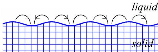
Fig. 1. Melting-freezing wave on the surface between fluid and solid phases.
